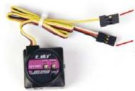
Connect the gyro with CH4
